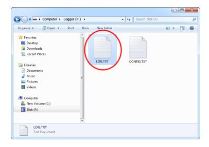
The removable disk will contain the file LOG.TXT with a text log of all captured data. The data is stored in the same format as appearing on the serial bus, without any encoding. The upstream data (TX) and downstream data (RX) will be differentiated by the channel headers interleaved in the log file. The *AirDrive RS-232 Recorder* will also interleave time-stamps. The file LOG.TXT can be viewed and searched with any text editor, such as *Notepad* or *MS Word*.
