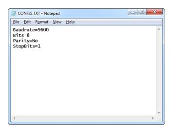
Replace *Baudrate* with the actual baud rate in bits per second of the serial bus you want to log data from. Replace *Bits* with the number of bits per transfer (5...8). Provide the parity check using one of the following strings: *No, Even, Odd, Space*, or *Mark*. Replace *StopBits* with the number of stop bits per transfer (1, 1.5, or 2).
