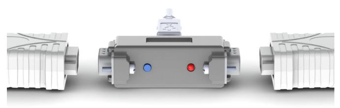
The device may be powered from a standard USB port. Alternatively, an external +5V DC (min. 200 mA) power supply may be used to power the device through the USB port (cell phone chargers with USB connectors are well suited for this).
