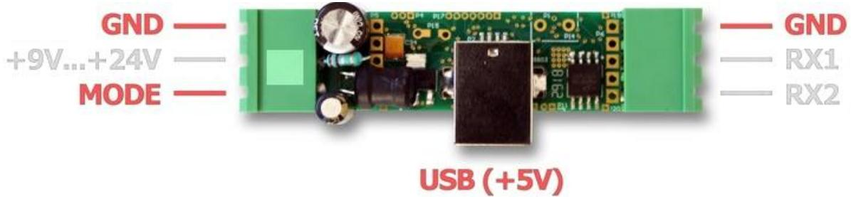
After a few seconds, the device will automatically get detected as a mass storage device, and pop up as a removable drive.
