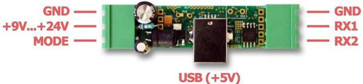
The device may be powered from a standard USB port with +5V DC. Alternatively, an external +9...+24V DC (min. 200 mA) power supply may be used to power the device. It is important to connect the ground of the monitored bus to the *SerialGhost's* ground connector GND.
