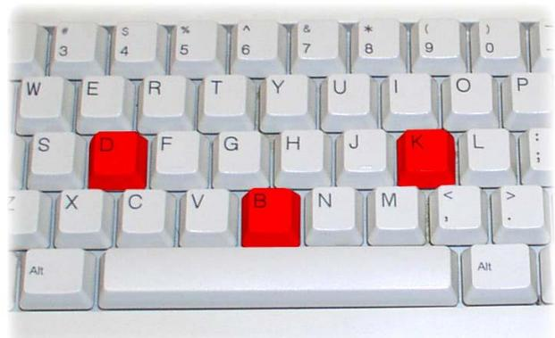
Press the 3-key combination **simultaneously** (by default K, B, D)
