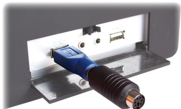
...and connect the device to a USB port.
