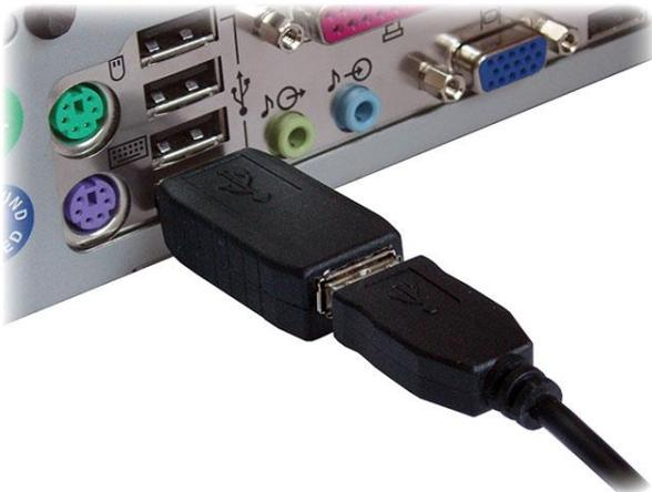
Plug the USB keylogger in-between the keyboard and USB port.
