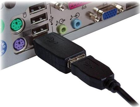
Plug the USB keylogger in-between the keyboard and USB port.
