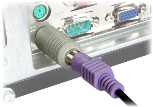
Plug the PS/2 keylogger in-between the keyboard and PS/2 port.
