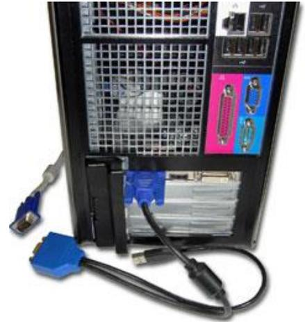
Then, connect the output device (TV or monitor) to the other end of the *VideoGhost*. Finally, connect the USB connector to a free USB port.
