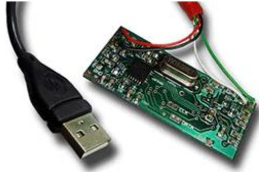
*Receiver circuit board wired to USB*
