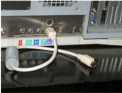
*Connect the transmitter unit to the PS/2 port*
