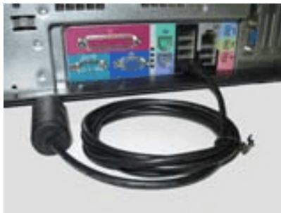
*Connect the receiver unit to a free USB port*
