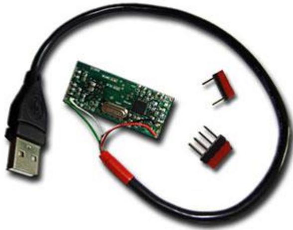
*USB cable and jumpers for SAM-BA bootloading*
