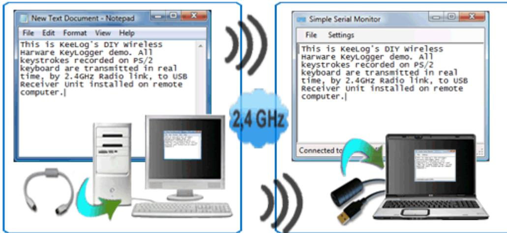
*Remote computer with PS/2 transmitter unit*
