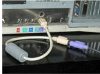
*Connect the PS/2 keyboard to the transmitter unit*
